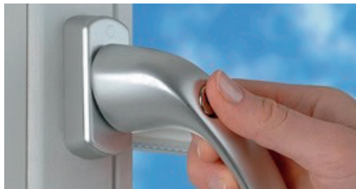
HANDLE WITH BUTTON to move the fitting, the button needs to first be pressed and then the handle turned. Like the Secustic® handle, it prevents windows from being opened from the outside
